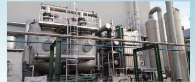
鞍山七彩化学 (活性炭吸附箱) Anshan Qikai Chemical (Activated carbon adsorption chamber)
